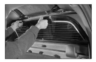
With the rear glass tilted at an angle, place the bottom edge in the lower channel of the window frame.
